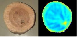
←Cross-sectional imaging (right) of a wooden log with a hole in it (left ) using ultrasonic time-offlight computed tomography. Content :
